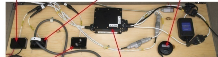
Data acquisition unit with CANbus connection
