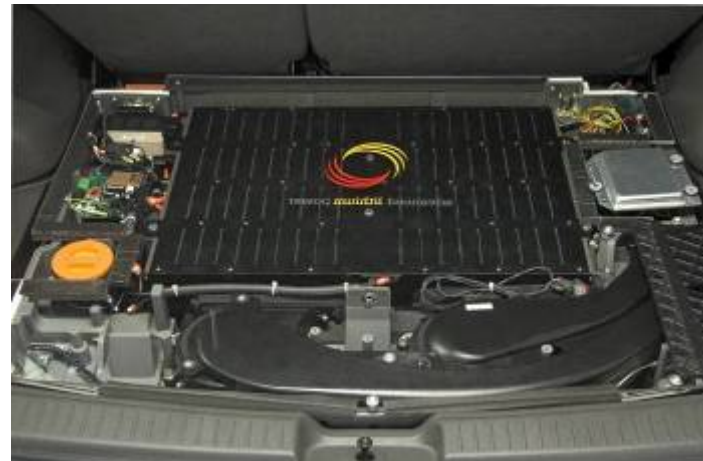
Lithium-ion Battery Pack Installed in Test Vehicle
